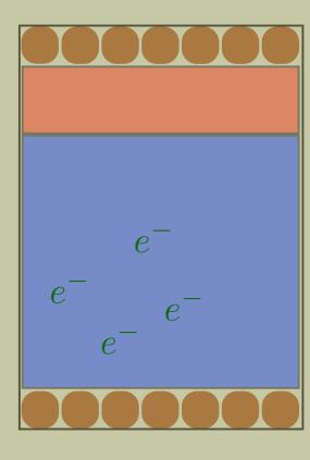
$Xe \rightarrow Xe^*, Xe^+$ produces photons and electrons Two types of signal: S1: prompt scintillation S2: proportional scintillation (from ionization) Signal (too small) **S**2 **S1**
